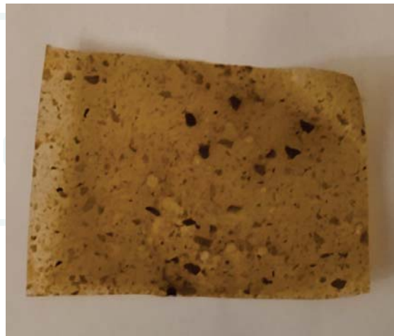
photo by: UNS team (Flexible Sample for Mechanical Testing of Mushroom Based Substrate)
